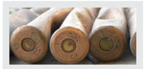
Sudanese 7.62 x 54R mm cartridges, manufactured in 2012, with headstamps 1\_54\_12
