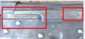
Type 56-1 with marks removed by grinding
