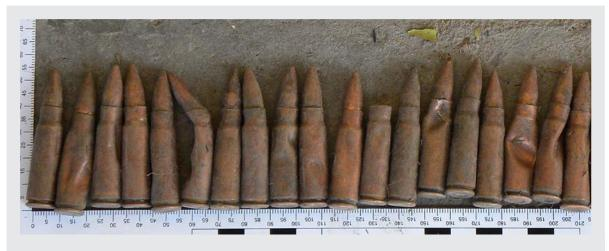
$7.62 \times 39 \text{ mm}$  ammunition, visibly damaged, consistent with sudden impact as a result of airdropping
