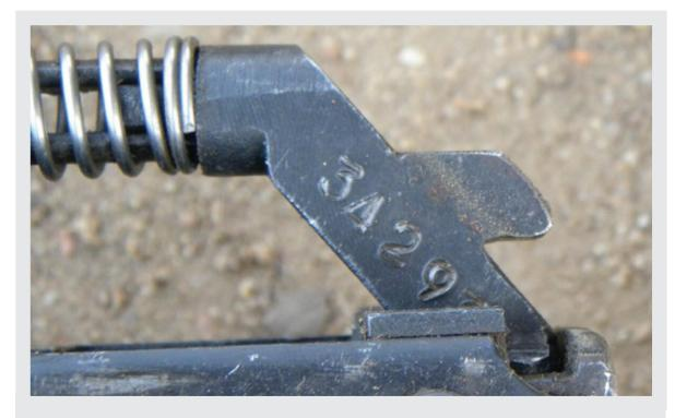
Partial repeat of the serial number (34293) on recoil spring guide
